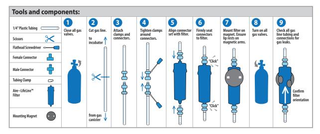
Figure 1: Tools / supplies and directions needed for proper installation of the Aire~LifeLine
