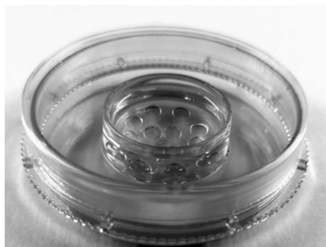
FIG. 1. The Humdish, with 20 \mu L medium drops covered with 3 mL mineral oil.
