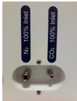
Figure 11.1 Gas inlets on the back of Mini MIRI® Dry and MIRI® Humidity multiroom IVF incubators
