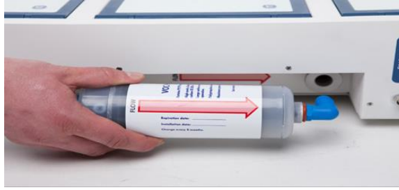
Figure 12.2 The way of pulling filter
