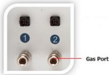
Figure 25.1 Gas sample ports
