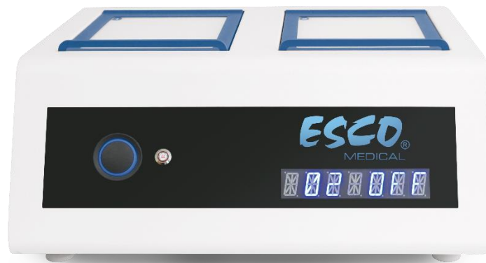
Figure 7.1 Compartment numbers on Mini MIRI® Dry and Mini MIRI® Humidity multiroom IVF incubators
