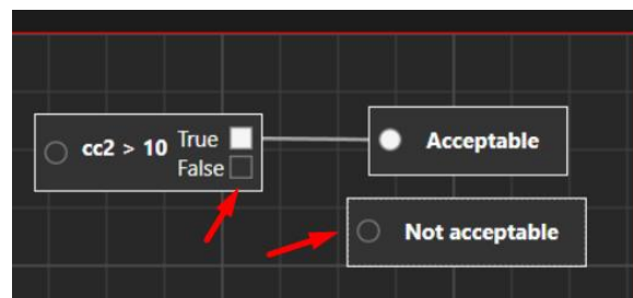
Figure 7.130 Conditional node with connected “Acceptable” result node
