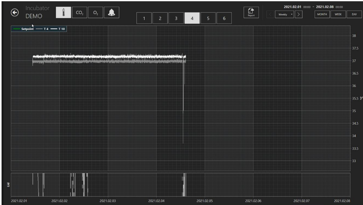
Figure 7.103 “DEMO” incubator temperature incubation data log view
