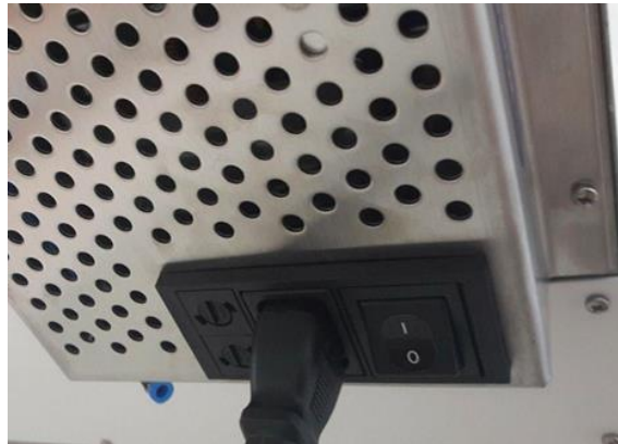
Figure 34.10 Power button on the back of the Multi-zone ART Workstation
