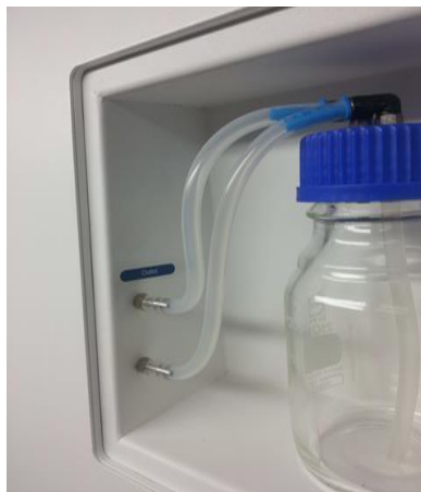
Figure 11.5 Tubes connected to the flask
