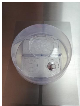
Figure 11.8 Gas hood placed over the gas nozzle
