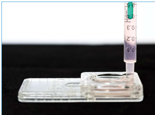
Figure 6. Slowly aspirate a maximum of 500µL.
